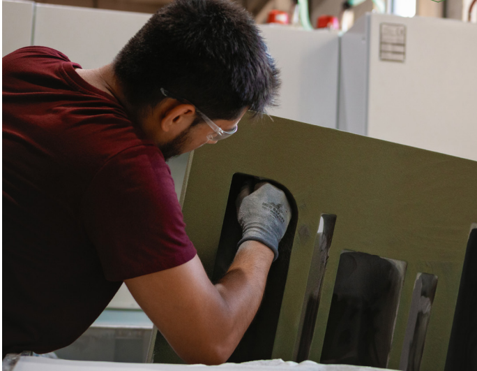
A large print is removed from the sand print bed, left, of the S-Max sand 3D printing system at Kore Mart, right
